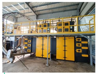
High-efficiency sludge dryer
